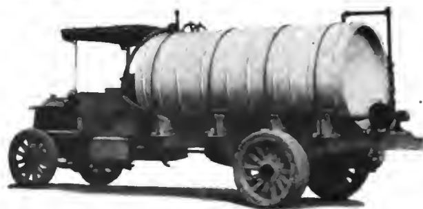
Upper—Packard 3-ton truck chassis equipped with a tank body, used by the Brooklyn Union Gas Co., Brooklyn, N. Y., to pump water out of gas lines
